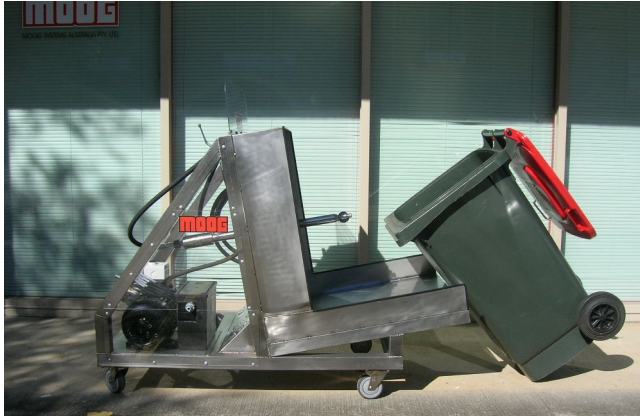
Bin in loading position.
