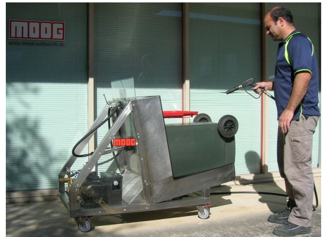
Use of high pressure lance for cleaning outside of bin.
